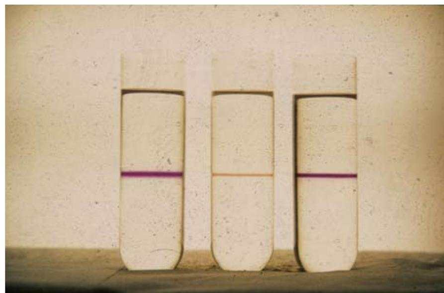
Materials. Centrifuge tubes with fractions of cell membranes prepared as material for experimentation. Left, the purple membrane isolated from Halobacterium; centre, membrane depleted of pigment; right, a synthetically reassembled purple membrane.
