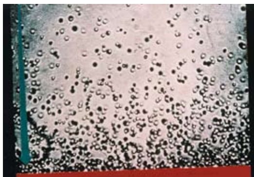
Microphotograph of the height distribution of resin granules suspended in water. Brownian motion is responsible for the statistical stability of this distribution, which is comparable to the height distribution of gas molecules in the atmosphere. This photograph was exhibited in the museum Jean Perrin helped create, the Palais de la Découverte, in the section dedicated to his own researches on Brownian motion. Phototèque Palais de la Découverte
