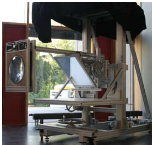
Experimental Historical Camera Obscura. A research tool for historians of art and science who investigate the 17th-century camera obscura. Designed and constructed for the MPIWG by Carsten Wirth and Henrik Haak
