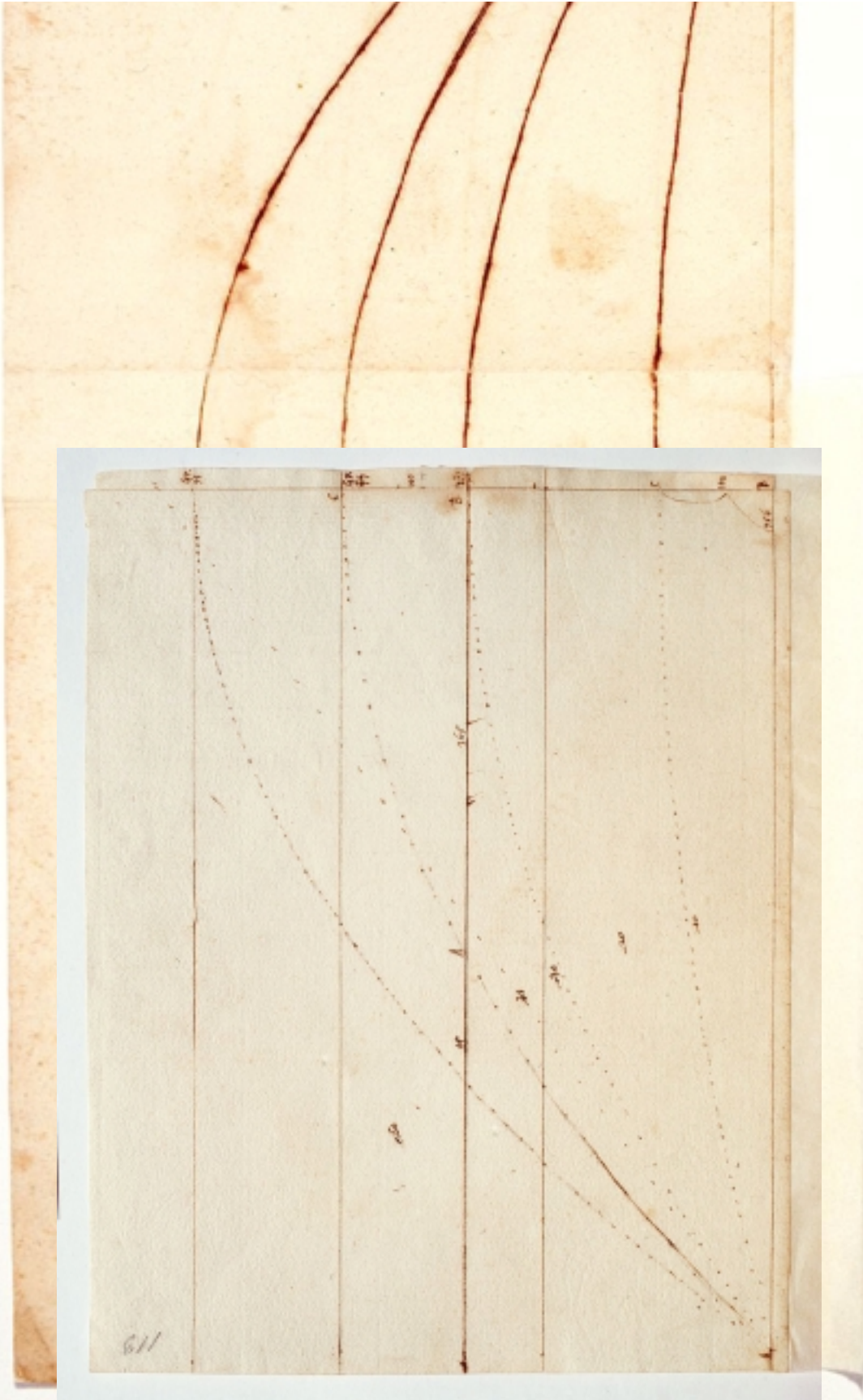
Figure 2. Ms. GAL. 72, FOLIO 41/42 (FOLIO IN THE BACK) USED AS A TEMPLATE FOR DRAWING PROJECTILE TRAJECTORIES ON FOLIO 113 (FOLIO IN FRONT)
