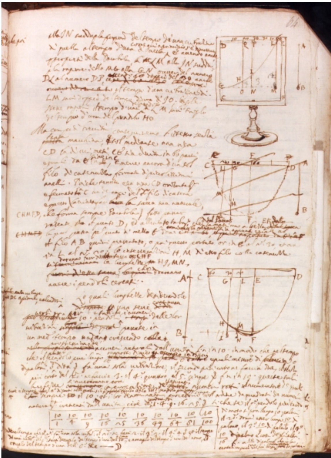
Figure 23. VINCENZIO VIVIANI'S APPLICATION OF A HANGING CHAIN FOR DETERMINING THE LENGTH OF A PENDULUM WITH A GIVEN TIME PERIOD
