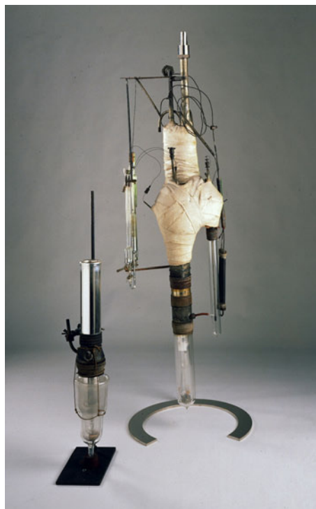
Figure 7: Kamerlingh Onnes helium liquefactor (courtesy of Museum Boerhaave, Leiden).
