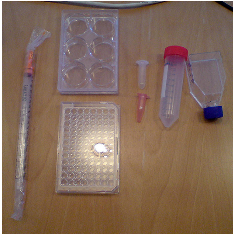
Figure 14: Single use, disposable plastic labware and sample containers, straw pipette, two microwells, two pipette tips, urine sample container, stackable culture flask. Medicinsk Museion Collection, Copenhagen. (Courtesy of Medicinsk Museion Collection, Copenhagen, photo: Martha Fleming).
