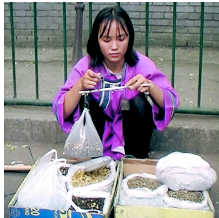
Moving the counterpoise of a Chinese steelyard.
