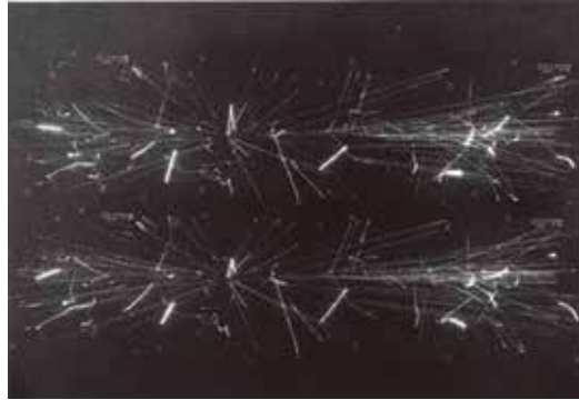
One of the first pictures of a 540 GeV proton-antiproton collision, as recorded in the big streamer chambers of the UA5 experiment at the CERN Super Proton Synchrotron in 1981. Courtesy of CERN Archive.
