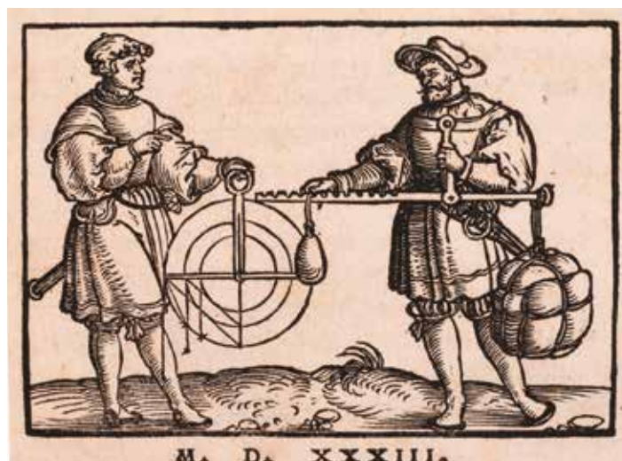
Title vignette of Apianus’ edition of Jordanus’ Liber de ponderibus displaying a scholar and a practitioner. The scholar explains the functioning of a steelyard according to Aristotelian principles.
