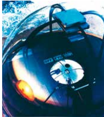
All-sky camera designed during the IGY to photograph active aurora bands. From: Robert H. Eather, Majestic Lights. The Aurora in Science, History, and the Arts , Washington (1980), p. 176.
