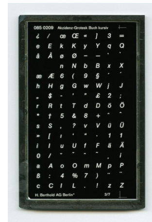
Fig. 3. Photo-typesetting matrix, Akzidenz-Grotesk. Since the early 1980s, type designers around the world have produced several other digital versions of Akzidenz-Grotesk under their own product names to avoid trademark issues. Printers and typographers appreciate these products and are well able to spot their similarities to the “original” font. SDTB / Photo: C. Kirchner
