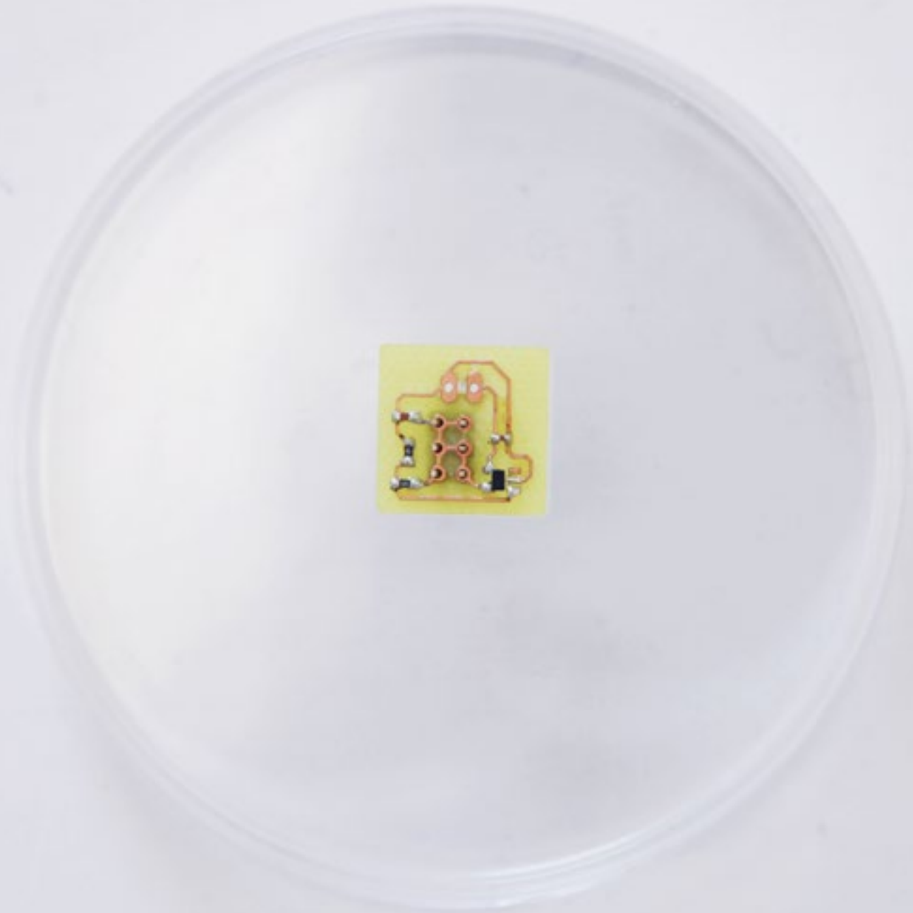
Electronic Plates Modified petri plates that provides electro-stimulation to culture.
