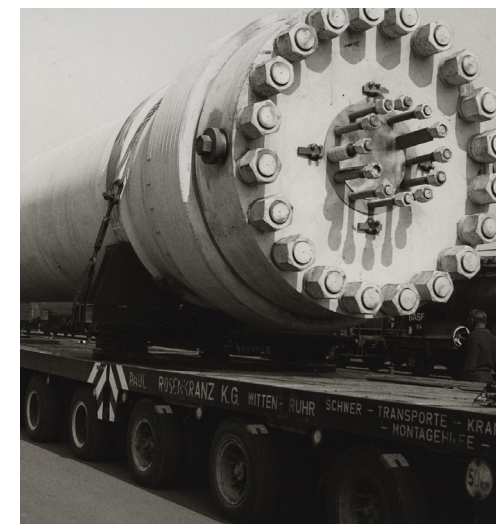
02 Transporting a high-pressure ammonia reactor (oven) in 1969. The size of the pipes had remained similar since Haber's invention was upscaled 60 years earlier. Source: BASF SE, Corporate History, Ludwigshafen.
